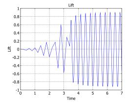
Figure 6-2: Time evolution of the total lift force on the cylinder.
