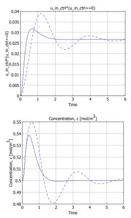
Figure 9-2: PID-controlled inlet velocity (top) and concentration in the measurement point (bottom) as a function of time for  $k_{\rm P}=0.5~m^4/({\rm mol\cdot s})$  (solid) and  $k_{\rm P}=0.1~m^4/({\rm mol\cdot s})$  (dashed).
