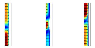
Figure 10-15: Snapshots of the velocity field and the shape of the inside of the tube at t = 0.3 s, t = 0.7 s, and t = 1.2 s. The colors represent the magnitude of the velocity, and the arrows its direction.
