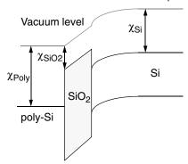
Figure 12-6: A band diagram of the MOS material system. The necessary parameters to align the materials are the affinities of the oxide and semiconductor, plus the work function of the polysilicon gate, which this model assumes has the same properties as aluminum
