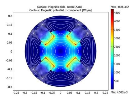
Figure 4-8: The magnetic field density and flowlines in the center of one of the quadrupole magnets.
