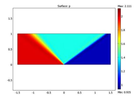
Figure 6-13: The pressure distribution in the shock tube. The y-axis represents time.
