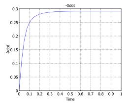
Figure 6-5: Falling velocity (m/s) of the grain versus time. After the solution time of 1 s, the velocity approaches the terminal velocity.
