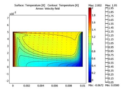
Figure 10-11: Marangoni convection with a temperature difference of 2 K.
