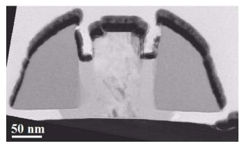
Cross-section TEM (transmission electron microscope) image of a 70-nm MOSFET fabricated in the clean room at the Royal Institute of Technology in Kista, Sweden (a project of P.-E. Hellström and others).
