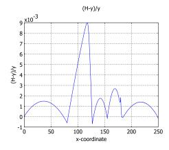
Figure 7-3: Fractional error in water table geometry computed using hydraulic head predicted by COMSOL Multiphysics, H, and water table elevation, y.
