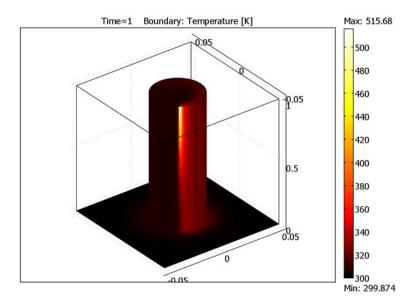
Figure 8-4: Temperature distribution after 1 s of laser heating.
