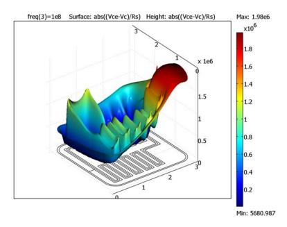
Figure 12-4: The harmonic part of the collector current density at 100 MHz.
