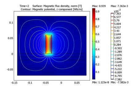
Figure 10-6: Magnetic vector potential and magnetic flux density, B field (white areas surpass the plot color range).
