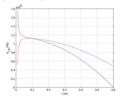
Figure 5-1: Radial (blue) and azimuthal (red) stress components in a homogeneous flywheel of constant thickness.
