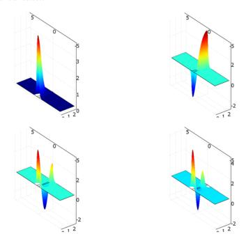
The four lowest electronic-energy levels for the case l = 0.
