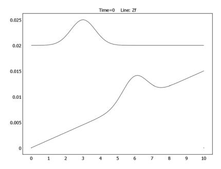
Figure 5-15: The initial water surface profile,  $z_0 + z_f$ , and the sea bed profile,  $z_f$ .
