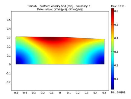
Figure 6-16: Velocity field inside the tank at t = 6 s.
