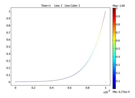
Figure 8-6: Relative laser-beam intensity as a function of sample depth.
