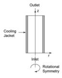
Figure 3-5: Geometry for the 2-dimensional rotationally symmetric models.
