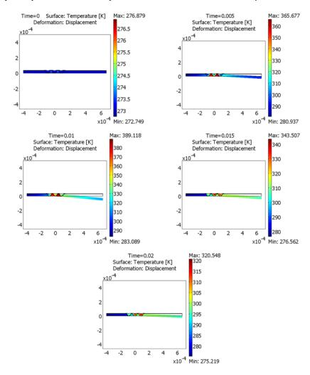
The animation shows how the temperature in the robot leg increases and how it bends downward, as expected. Note that the temperature should be interpreted as a deviation from the initial state, which is room temperature. After 10 ms, the power is turned off,
