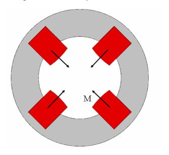
Figure 4-6: Cross-sectional view of one of the magnetic quadrupoles used in the lens.
