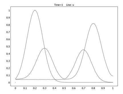
Figure 5-24: Shape of the pulse at t = 0, 0.5, and 1:  $\alpha + \beta = 0.5$ .
