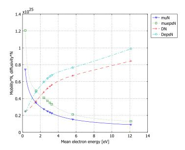
Figure 5-32: Transport properties calculated using the two-term Boltzmann equation.
