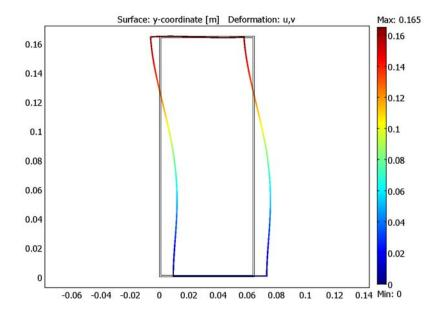
Figure 10-13: The deformation (exaggerated) of the container filled with gas.
