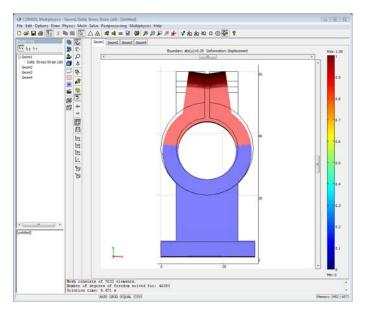
Figure 13-6: Clamp deformation due to the screw force.
