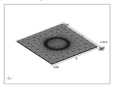
Figure 8-3: The 3D mesh produced by extruding a 2D triangular mesh, refined along the circular laser incident line.
