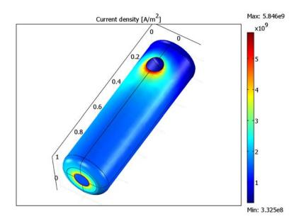
Figure 5-19: Local magnitude of the electric current density  $(A/m^2)$ .
