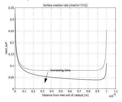
Figure 3-4: Surface reaction rate at the active surface. The largest reaction rate is obtained initially and is at the edges of the active surface. The reaction process almost reaches steady state at 0.5 s.
