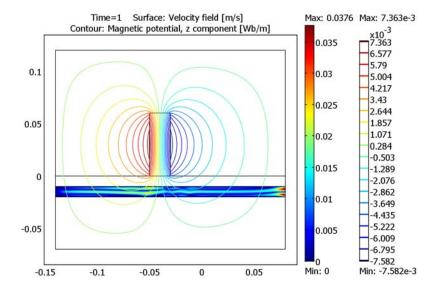
Figure 10-8: Velocity field at zero blood throughput (t = 1).
