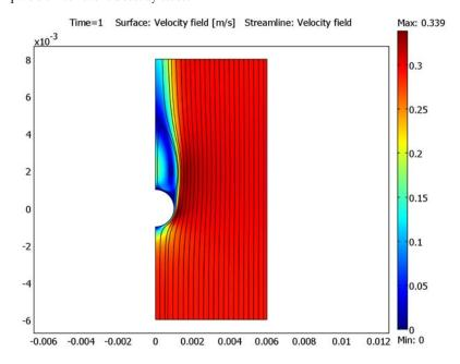
Figure 6-3: The velocity field at steady state. Note that the velocities are plotted in the reference system of the sand grain.
