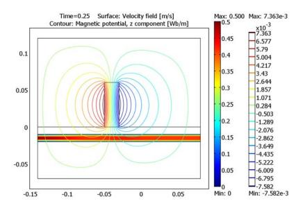
Figure 10-7: Velocity field at maximum blood throughput (t = 0.25).
