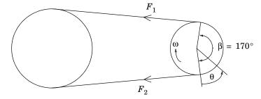
Figure 13-16: Pulley and driving belt with the external forces  $F_1$  and  $F_2$ .
