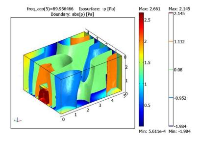
Figure 2-5: The sound pressure distribution for  $\omega = 569$  rad/s. The (negative of) the real part of the pressure is visualized as an isosurface plot, and the absolute value of the pressure as a boundary plot.
