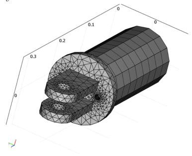
Figure 13-14: Finite-element mesh of the diagonal mounting assembly.
