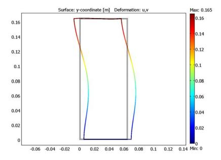
Figure 10-12: The deformation (exaggerated) of the container filled with milk.
