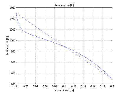
Figure 5-9: The temperature distribution with radiation (solid line) and without radiation (dashed line).
