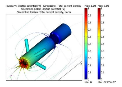
Figure 4-4: The plot shows the electrostatic potential distributed on the surface of the electrode. The total current density is shown as streamlines.
