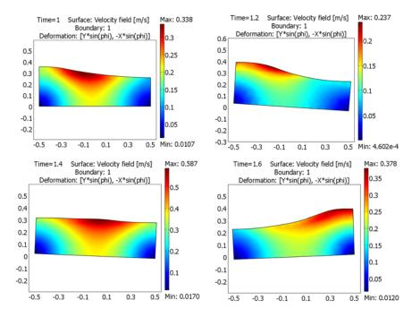
Figure 6-15: Snapshots of the velocity field at t = 1 s, t = 1.2 s, t = 1.4 s, and t = 1.6 s. The inclination of the gravity vector is indicated by the leaning of the tank.
