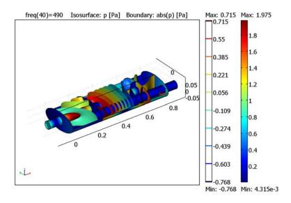
Figure 2-4: The solution at 490 Hz. The real value of the pressure is plotted as isosurfaces, and the absolute value of the pressure is displayed as a boundary plot on the inner walls of the muffler.
