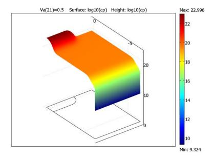
Figure 12-10: The hole concentration at 0.5 V forward bias.
