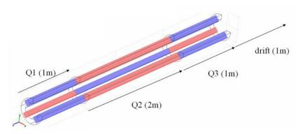
Figure 4-7: Cutout of the quadrupole lens. The second quadrupole (Q2) has its polarities reversed compared to O1 and O2. After traveling through the lens, the ions are left to drift 1 m.
