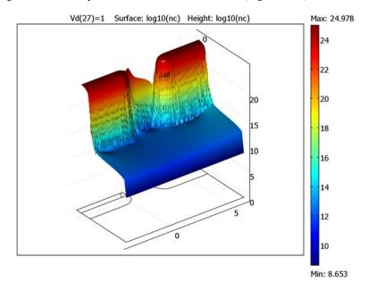
Figure 12-9: The channel close to the interface becomes visible in an electron-concentration plot. Notice the sharp drop in the channel concentration close to the drain contact, which is responsible for the saturation of the drain current.
