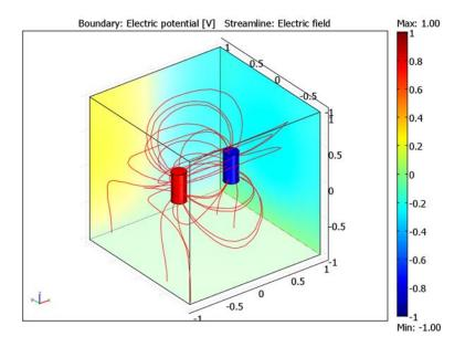
Figure 4-1: The electric potential (surface) and the electric field (streamlines).
