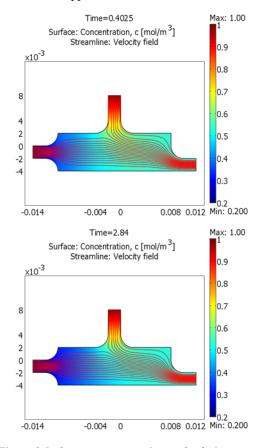
Figure 9-1: Oxygen concentration and velocity streamlines after approximately 0.01 s (top) and 1.5 s (bottom).
