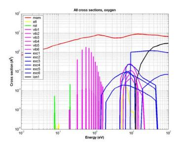
Figure 5-28: Electron-impact cross sections for molecular oxygen.
