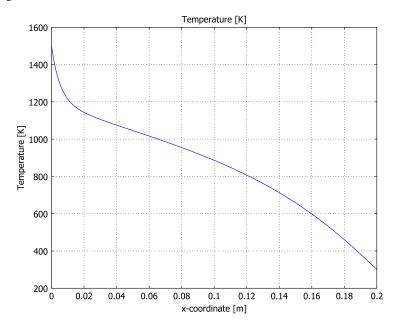
Figure 5-8: Temperature distribution along the pipe at t = 3600 s.
