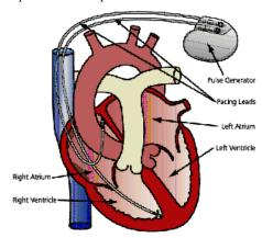
Figure 4-2: Schematic drawing of the heart with two pairs of pacemaker electrodes.
