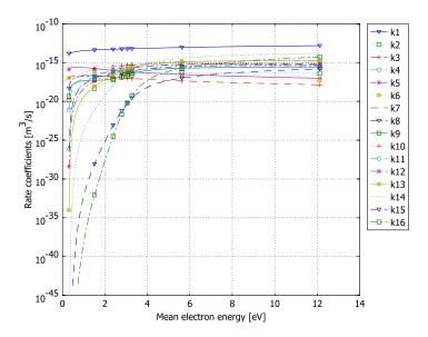
Figure 5-31: Rate coefficients calculated using the two-term Boltzmann equation.
