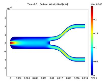
Figure 6-8: Velocity field when the valve is completely open.
