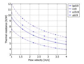
Figure 8-10: Thermal resistance as a function of the rate of air flowing over the heat sink.
