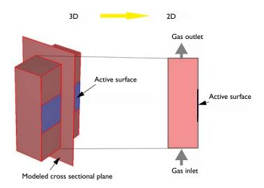
Figure 3-1: The modeled domain is a parallel plate reactor with an active surface where you want to model the concentration of surface species.
