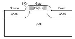
Figure 12-5: The model geometry. The simulation replaces the contacts with boundary conditions.
