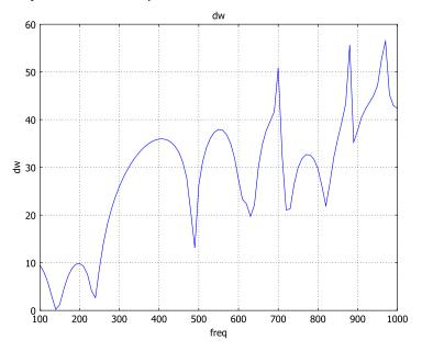
Figure 2-2: The damping (dB) in the muffler as a function of the frequency (Hz).
