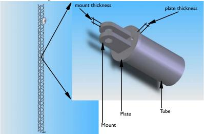
Figure 13-12: Mounting detail of a mast diagonal.
