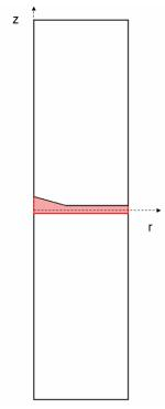
2D geometry of a perfectly cylindrical quantum dot and wetting layer.
