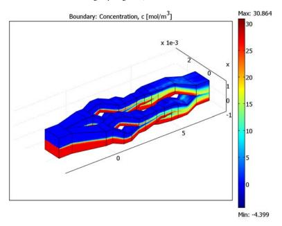
Figure 6-12: Following three split-reshape-recombine cycles, the outflow has eight fluid layers.
