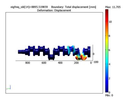
Figure 13-3: The twisting mode of the crankshaft throws.
