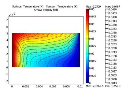
Figure 10-10: Marangoni convection with a temperature difference of 0.05 K.
