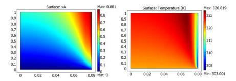
Figure 3-6: Conversion (left) and temperature (right) in the reactor.
