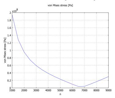
Figure 13-20: von Mises stress as function of rotational speed at point (0.019, 0.054).
