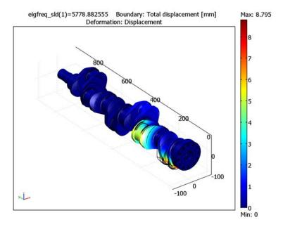
Figure 13-1: The first torsional mode in the crankshaft.
