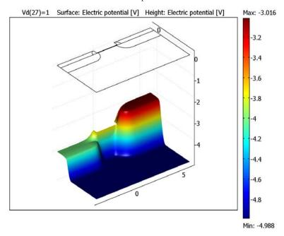
Figure 12-8: Surface plot of the electrostatic potential inside the MOSFET.
