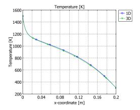
Figure 5-11: The temperature distributions from the 1D model (square markers) and the 3D model (triangle markers).
