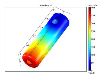
Figure 5-17: Electric potential distribution across the surface (V).
