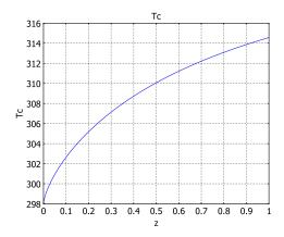
Figure 3-7: Coolant temperature along the length of the reactor.
