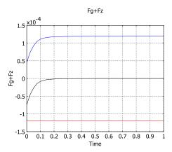
Figure 6-6: The forces on the sand grain. The force that the water exerts on the sphere (upper line) increases as the grain gains speed. The gravity force (lower line) remains the same, and the total force (middle line) tends toward zero as the solution approaches steady state.
