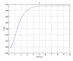
Figure 5-23: Time evolution in the center of a pellet with radius  $R_p = 2.5$  mm.
