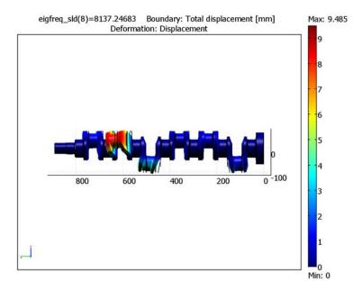
Figure 13-2: The bending mode of the crankshaft throws.
