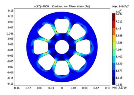
Figure 13-19: von Mises stress distribution at n = 9000 rpm.
