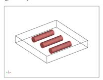
Figure 8-8: The heating device consists of three heating elements embedded in an aluminum block.
