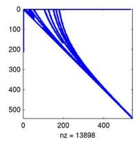
Figure 5-33: Sparsity-pattern plot of the assembled Jacobian matrix. The far off-diagonal elements are a result of the nonlocal couplings.
