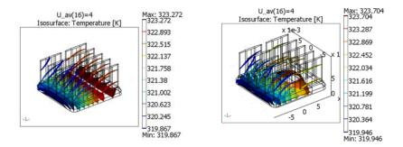
Figure 8-11: Temperature distribution in the standalone model of a lpd19 heat sink and in the model merged with the heating device (right).
