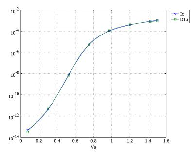
Figure 12-12: The green line with squares show the IV characteristics of the equivalent circuit, the blue line with triangles is that from the COMSOL Multiphysics Model Library model semiconductor\_diode.
