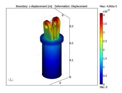
Figure 13-15: Deformed shape and boundary plot of the axial displacement for the mounting assembly with an end-plate thickness of 12 mm and mount thickness of 15 mm.
