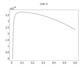
Local radial displacement, u, over radial coordinate, r, for constant flywheel thickness.
