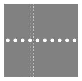
Figure 10-2: Using symmetry to reduce computation time and complexity. The model describes one section of the array of heating tubes (indicated by the dashed lines).
