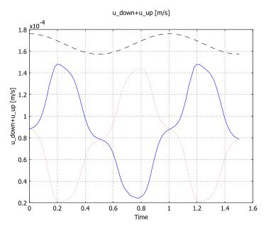
Figure 6-10: The blue line (solid) shows flow rate in the upper branch as a function of time, while the dotted line shows the flow rate in the lower branch. The dashed line shows the sum of the flow in the two branches.
