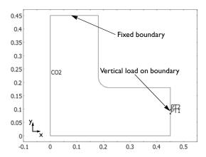
Figure 13-8: Geometry of the structure with loads and constraints.
