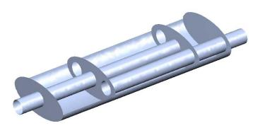
Figure 2-1: The geometry of a muffler. The exhaust fumes enter through the left pipe, pass the three resonator chambers, and exit through the right pipe.
