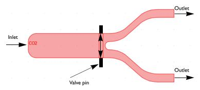
Figure 6-7: Depiction of the geometry and the operation of the fluid valve. Flow enters from one inlet at the left, but can leave the valve through two outlets at the right. The choice of outlet depends upon the position of the valve pin. In this model, two valve pins oscillate between the following positions: in front of one outlet channel to in front of the other. Sometimes flow is possible through both outlets, depending on the position of the pins.
