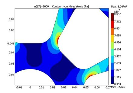
Figure 13-21: Von Mises stresses in a part of the pulley evaluated using accurate derivative recovery.
