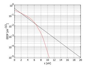
Figure 5-29: EEDF for an oxygen plasma calculated using the Maxwellian approximation (black) and the two-term Boltzmann equation (red).
