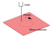
Figure 8-1: A moving laser heats a thin silicon substrate.
