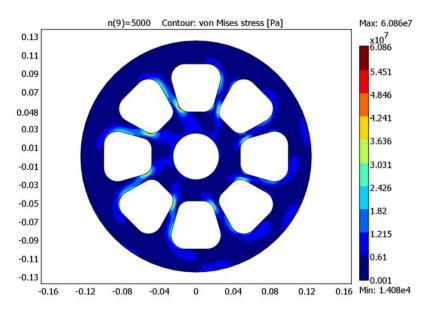
Figure 13-18: von Mises stress distribution at n = 5000 rpm.
