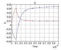
Figure 12-2: Turn on in 100 ns, where the red curve is the base current and the blue curve is the collector current.
