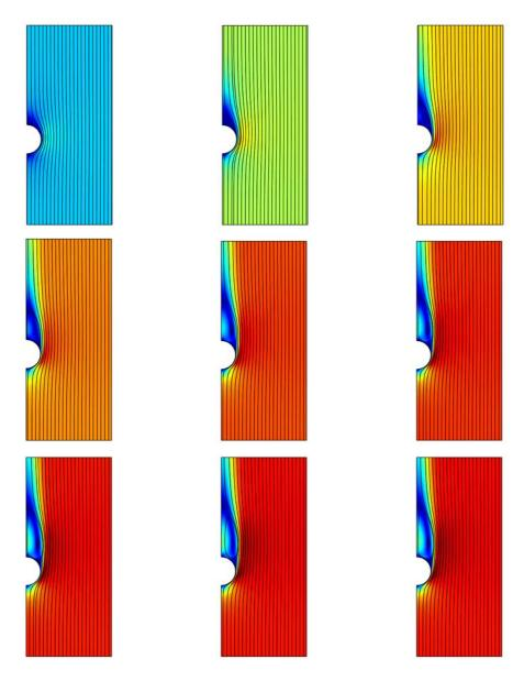
Figure 6-4: The velocity field around the sand grain at a series of times (t = 0.025 s, 0.05 s, 0.075 s, 0.1 s, 0.15 s, 0.2 s, 0.3 s, 0.5 s, and 0.75 s). For a color legend, see Figure 6-3.
