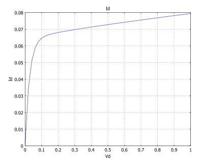
Figure 12-7: Drain current as a function of drain voltage for  $V_{\rm GS}$  = 0.8 V. Note that  $R_{\rm on}$  is 1/(slope of the curve) at the point where  $V_{\rm DS}$  = 0, which falls at the far left of the curve.
