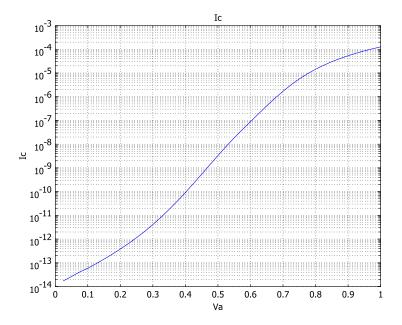
Figure 12-11: The IV characteristics of the semiconductor diode plotted in a logarithmic scale.
