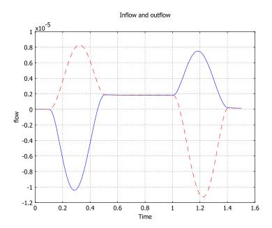
Figure 10-17: Inlet (blue solid line) and outlet (red dashed line) flow in  $m^3$ /s as functions of time. Positive values indicate that the gas is flowing in through the inlet and out through the outlet.
