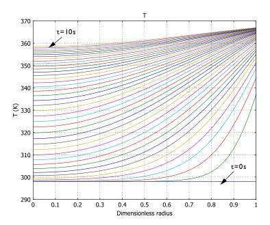
Figure 5-21: Temperature profiles from t = 0 to t = 10 s.
