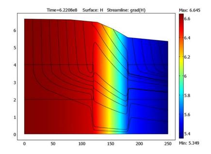
Figure 7-2: COMSOL Multiphysics estimates of hydraulic head and flow lines. The solution reproduces the results in Ref. 2.
