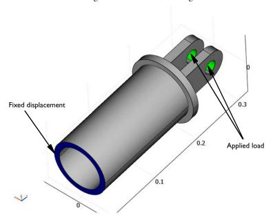
Figure 13-13: Boundaries with constrained displacements and applied loads.
