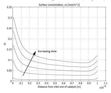
Figure 3-3: The concentration of adsorbed species increases with time. The edge effect appears at both edges due to the increased supply of reactants. This figure displays the concentration after 0.05, 0.5, 1.0, 1.5, and 2.0 s.
