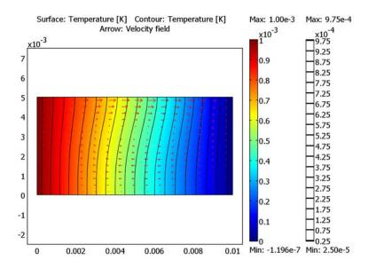
Figure 10-9: Marangoni convection with a temperature difference of 0.001 K.
