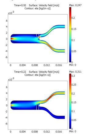
Figure 6-9: Velocity field when the valve is half way closed from above (top) and fully closed from below (bottom).
