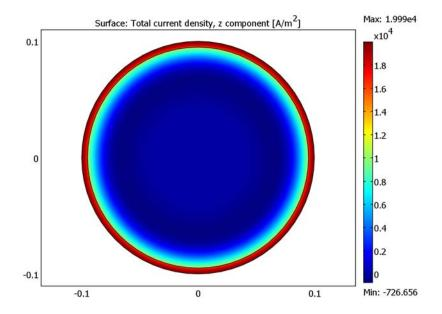
Figure 4-5: Total current density through a wire carrying an AC current.
