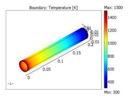
Figure 5-10: 3D temperature distribution in the pipe.
