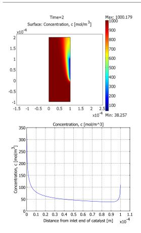
Figure 3-2: The concentration of the reacting species, c, after 2 seconds of operation in the 2D cross section (top) and along the active surface (bottom).
