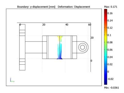
Figure 13-5: Maximum and minimum y-displacement at the center of the clamp cylinder.
