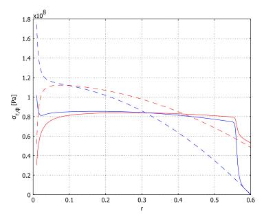
Figure 5-3: Radial (blue) and azimuthal (red) stress components for initial (dashed) and optimized (solid) flywheel profiles.
