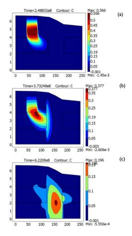
Figure 7-4: Plume concentrations calculated with COMSOL Multiphysics at three times: (a) t = 8 years, (b) t = 12 years, and (c) t = 20 years.
