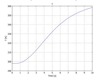
Figure 5-22: Time evolution of temperature in the center of a pellet with radius  $R_p=5\ \mathrm{mm}$
