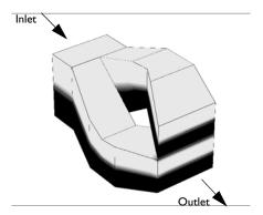
Figure 6-11: The micromixer splits the incoming fluid in the direction perpendicular to the interface separating the two fluid layers. After recombining them, the mixer stacks the two flows on top of each other, resulting in four fluid layers.
