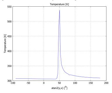
Figure 8-5: Temperature distribution along the laser-beam incident trajectory on the top surface after  $0.7\,\mathrm{s}$ .
