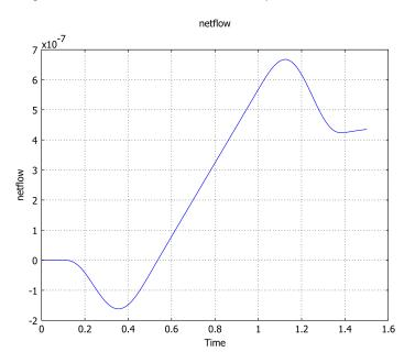
Figure 10-18: Accumulated flow (m<sup>3</sup>) through the pump versus time (s).
