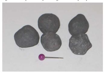
Figure 5-20: Hematite pellets after drying and oxidation (end product).
