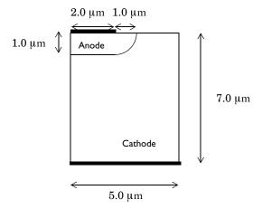
Thicker lines indicate electrical contacts. This example applies a potential  $V_{\rm a}$  to the anode, and the cathode is grounded.
