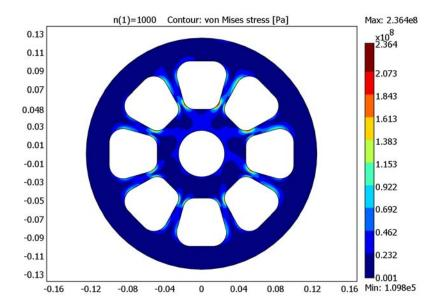
Figure 13-17: von Mises stress distribution at n = 1000 rpm.
