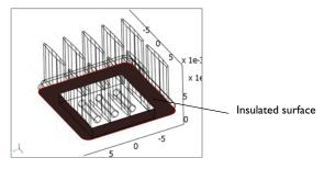
Figure 8-9: The surface is the part of the heat sink that is insulated.
