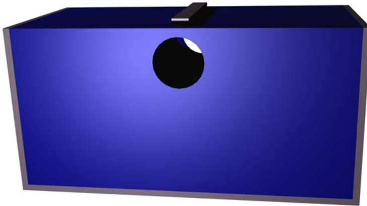
Figure 5-1: The electrode is placed on a conducting block with an air-filled cylindrical cavity inside.
