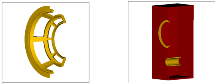
Figure 3-35: The frame and the vented enclosure.
