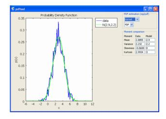
The fit of the histogram and parametric distribution, and the different moments, can be used to validate the chosen distribution.
