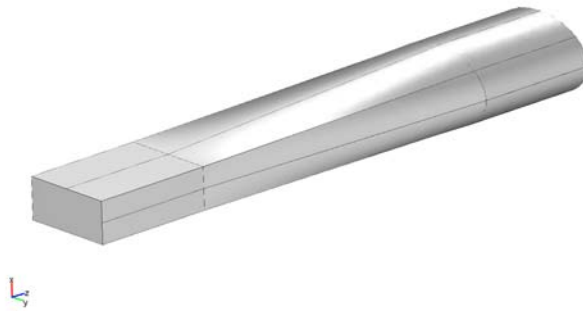
Figure 3-12: The geometry of the waveguide adapter.
