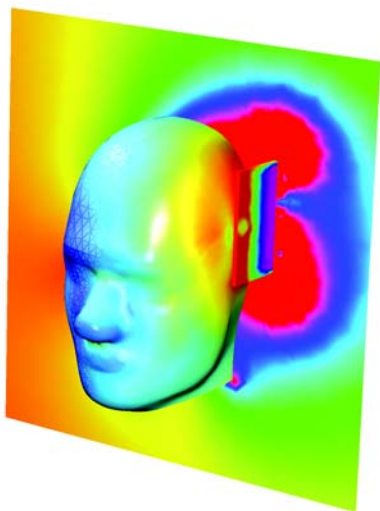
SAR simulation based on the radiation coming from a mobile phone in the RF Module. The model is available in the RF Module Model Library.
