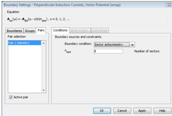
Figure 2-2: The Boundary Settings dialog box with sector antisymmetry selected for Pair 1.
