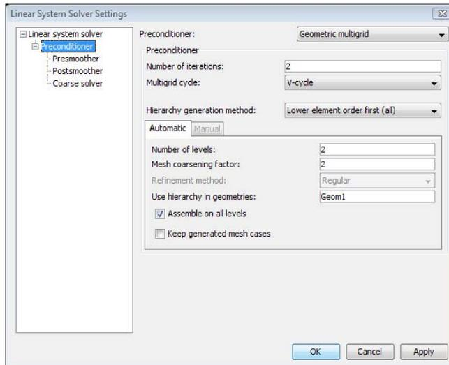
Figure 2-8: The multigrid settings for the GMG preconditioner.
