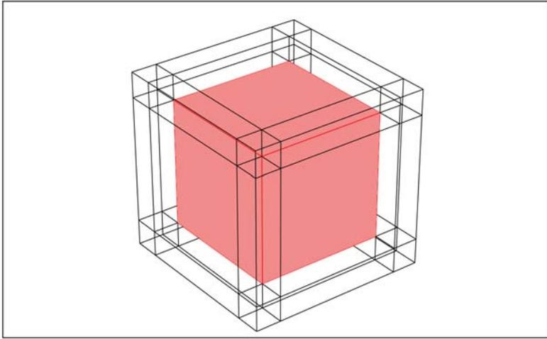
*Figure 2-4: A square surrounded by typical infinite-element regions of Cartesian type.*
