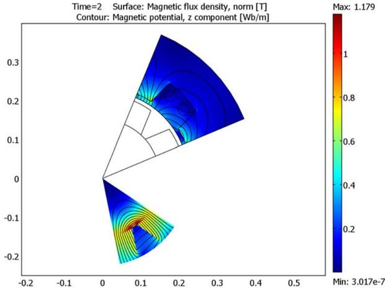
*Figure 2-3: The rotating sector has rotated more than half a revolution but is still coupled with the static sector.*
