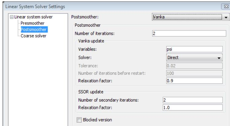
Figure 2-15: The postsmoothing settings (the figure shows only the upper part of the dialog box).
