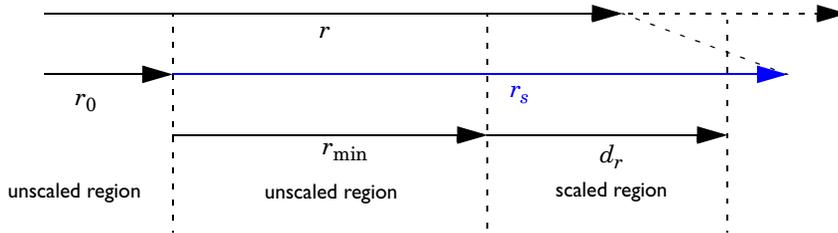
*Figure 3-1: The coordinate transform used for the mapped infinite element technique. The meaning of the different variables are explained in the text.*
