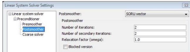
*Figure 2-11: The postsmoother settings (the figure shows only the upper part of the dialog box).*
