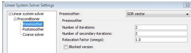
Figure 2-10: The presmoother settings (the figure shows only the upper part of the dialog box).
