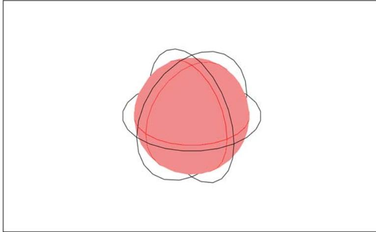
Figure 2-6: A sphere surrounded by a typical spherical infinite-element region.
