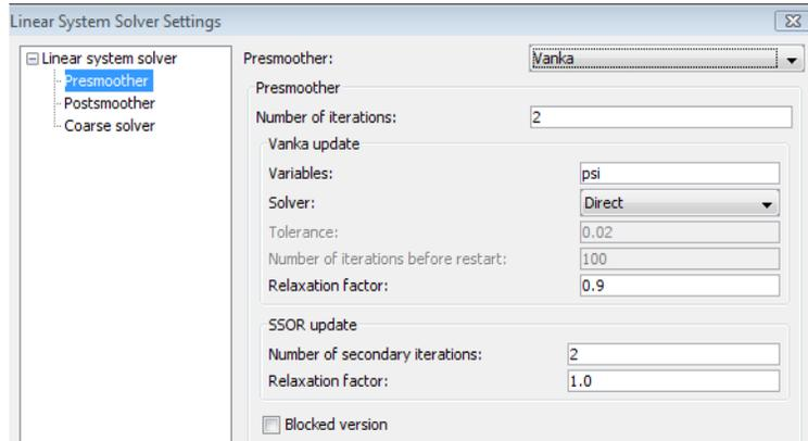
Figure 2-14: The presmoothing settings (the figure shows only the upper part of the dialog box).
