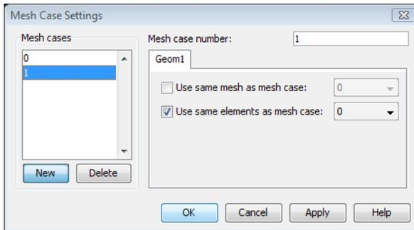
*Figure 2-9: Specifying the same mesh for both meshes in the Mesh Case Settings dialog box.*
