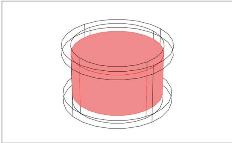
*Figure 2-5: A cylinder surrounded by typical cylindrical infinite-element regions.*
