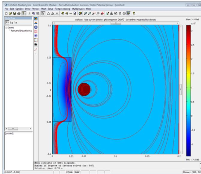
The plot shows the eddy currents induced in the cylinder and the constant current density in the coil.
