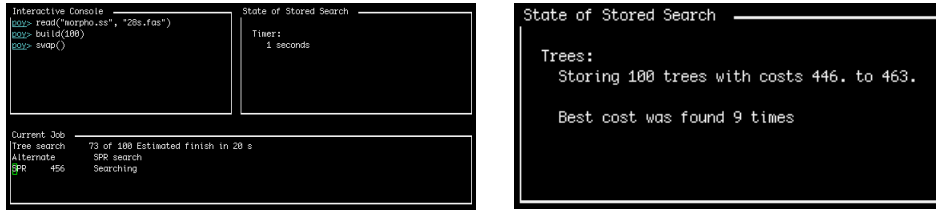
Figure 2.25: Performing a local search. When searching (left panel), the Current Job window reports the number of the tree that is currently being analyzed (73 of 100), a method of branch swapping (Alternate), a function being currently performed (SPR search), and a cost of the current tree (456). When the searching is finished (right panel), the State of Stored Search window displays the best (446) and worst (463) costs, the number of trees stored in memory (100), and the number of trees of the best cost (9) recovered from independent tree builds. Note these trees may not necessarily have unique topologies.
